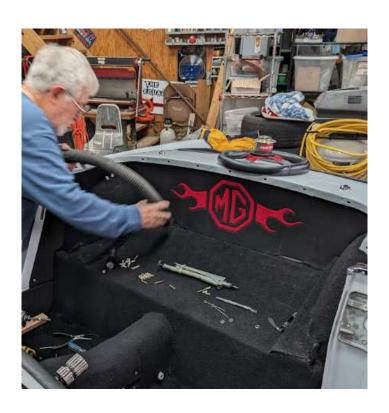
It took two of us to snake the custom-fitted partition into the channel built into the underside edge of the deck. Solidly TIGHT!
