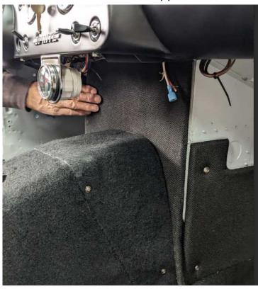
Side panels in footwells get extra care when locating the drill holes for screws so that panels may be removable. The big deal about drilling holes in the firewall and other locations in the footwells is MAINLY because drill bits can find important things that you didn't want poked or scraped, like fuel & brake lines or spendy equipment.
