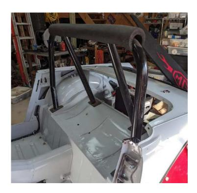
Nicely fitted roll bar. Almost as tall as height of car body, when properly fitted, prevents dents in delicate brain cases on those occasions when the wheels exchange places with the top.
