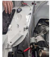
The battery cable takes special route to safely reach the starter, and a new cable connects starter to power block on firewall.
