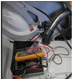
The battery box, along with the battery cables and the cutoff switch inside the trunk, are now mounted and ready for the battery.
