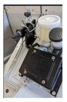
against metal walls to degrade the tight fit. A small internal leak means a master cyl replace, and recoupling of carefully bent steel lines & joints that weren't that eager to cooperate in the first place.
