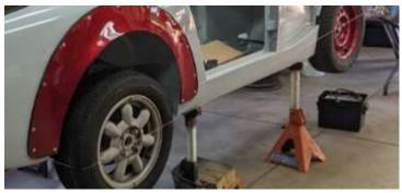
If you will look closely, you will find Hank's special Alignment Tool stretched across the tires from front to back. Hank wanted to make sure the body was resting squarely and in alignment with the car body, suspension, and wheels. He used a string! It tells you clearly if the body and the wheels are resting squarely in agreement with each other. Slick.
