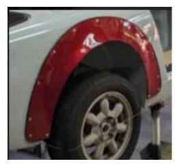
Prep & install of the mounts for the red flares brings its own set of complications. The flares are secured in place on the fenders for a perfect fit.
