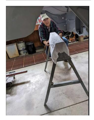
With the shell absolutely stable and solidly mounted on the sawhorses, the task of chasing all the threads on all the bolts & nuts & holes in the body can begin.
