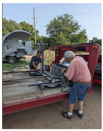
Hank makes sure all of the tie-downs at the front and rear are solid and taut to prevent too much sway. Ties must be flexible and not too tight, so that paint isn't chafed nor body metal is distorted.
