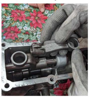
The new fixture is on the rod, below right, shows that it allows for more comfortable shifting positions, considerately well forward of original shift fixture envelope, allowing
