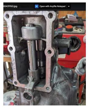
Do a check fit on the new gearshift fixture and lever and check the fit of universal.
