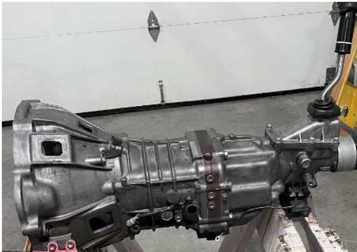
Below, the new JDM is fitted to new bell and the new shift lever shown installed.
