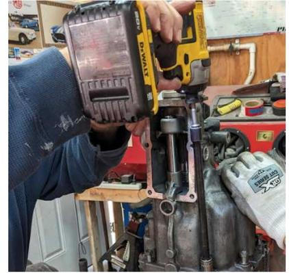
New speedo gears are carefully meshed and compressed into place.
