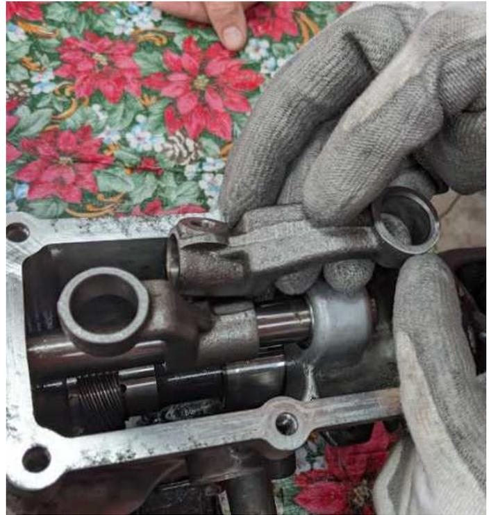
The new fixture is on the rod, below right, shows that it allows for more comfortable shifting positions, considerably well forward of original shift fixture envelope, allowing the driver to have easier operation of the gearshift knob.
