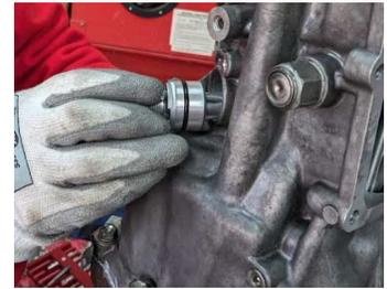
If speedo and gearing works well together, it's time to install the shifting tower.
