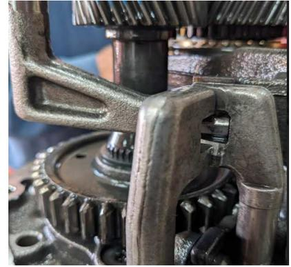
Seal is in; case goes back on and bolted down with very specific bolts with specific torques.
