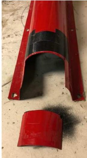
This was the most nerve-wracking bit: cutting off the rear transmission support with a reciprocating saw!
